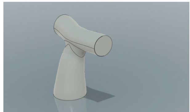
Fig.1 Development of preliminary CAD drawings to obtain the fluid domain of the geometry for the evaluation of pulmonary circulatory intervention with outflow tract reconstruction.
