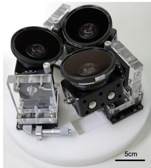
Figure 2. Three high-speed cameras for sequential image recording developed in the study; one sequence with two leaflets images from each pair of three cameras. The set of cameras was installed in the water-filled visualisation chamber. Images were monitored and synchronised via Wifi transmission.
