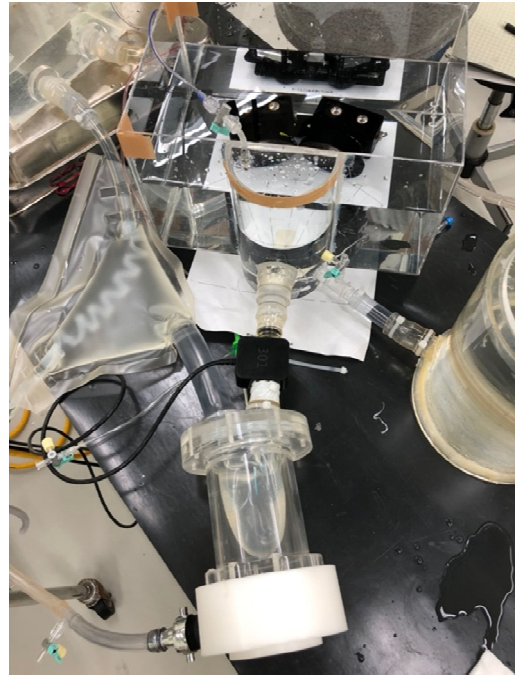
Figure 1. Whole view of the pulmonary arterial circulatory model. The high speed multi-angle images of the leaflets were synchronously obtained from the outflow position of the valve.
