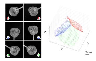
Figure 4. Processed images obtained by the three cameras (left) and the reconstructed leaflet images (right)
