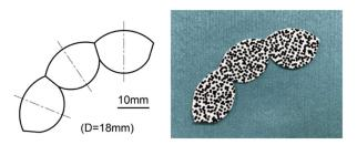
Figure 1. Schematic illustration of the fan-shaped leaflet for the 18-mm-diameter ePTFE valved conduit (left) and the valve leaflet membrane with speckle pattern transcribed for digital image correlation.
